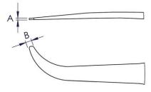
**Tip Dimensions:** A (tip thickness) 0,50 mm – 0,020 inch
